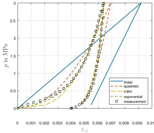
Fig. 1: Comparison of FE-simulations with different normal contact laws to experiments in [2] and [3] for compression tests of three stacked sheets.
