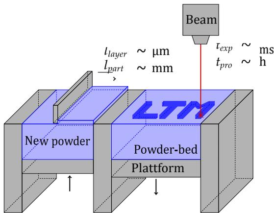
Fig. 1: Principle steps of powder bed-based AM processes
