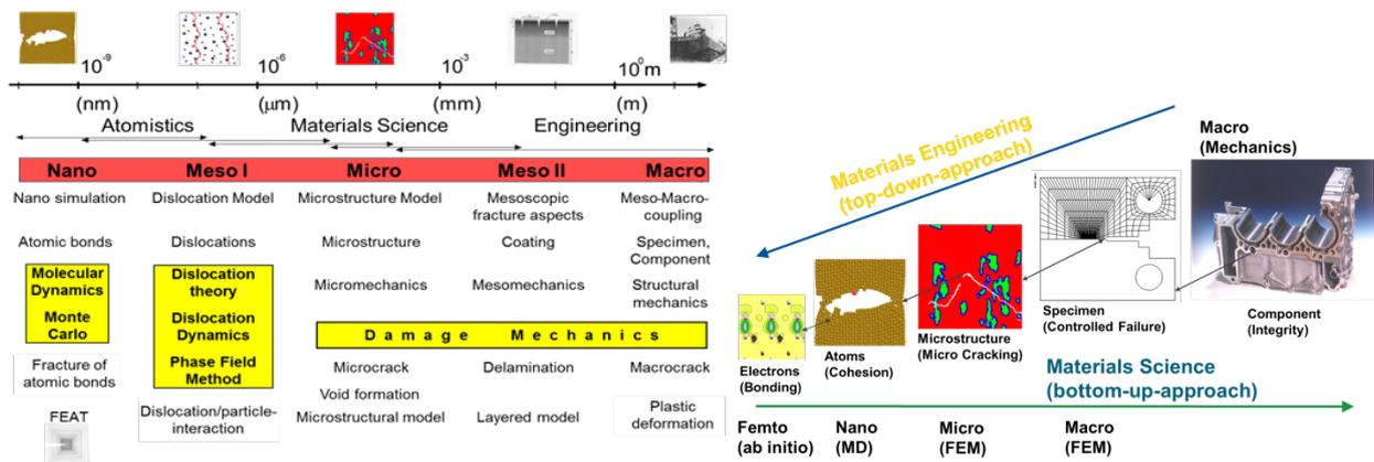
Figure 1. Multiscale Materials Modelling Figure 2. Scale Bridging Technique (MMM)
