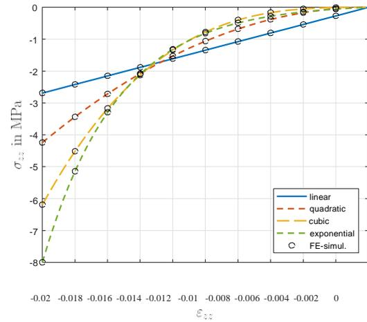
Fig. 2: Stress-strain curve of a representative volume element consisting of two half-sheets in contact for a numerical homogenization and the identified material mode.
