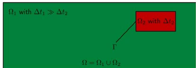
Fig. 2: Domain decomposition with heterogeneous time step size
